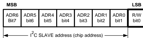
Figure 22. I 2 C Chip Address
